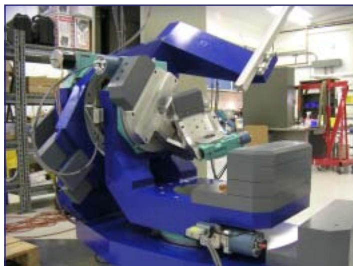
Figure 2. The new diffractometer, based on “kappa” geometry, has six independent rotation axes allowing virtually any reflection geometry.
