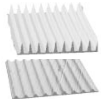
Figure 3. AFM images of micromachined corrugations on glass before (upper image) and after (lower image) annealing at 810°C. The thermal treatment has had a smoothing effect.
